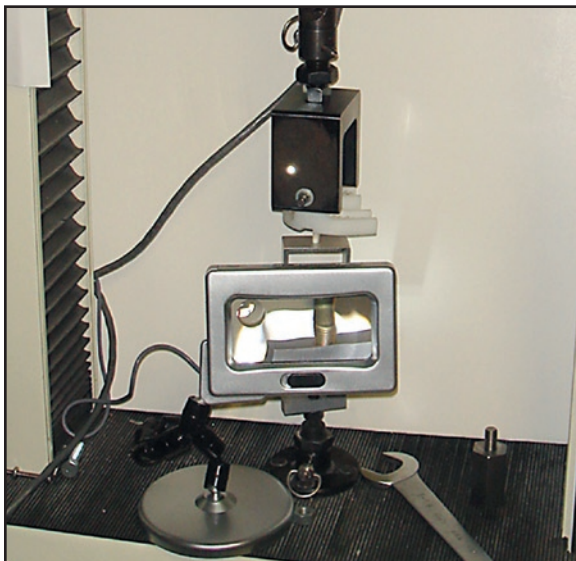
Fig. 2 Maxillary right first premolar and corresponding aligner secured to testing machine, and vertical force applied to dislodge aligner from tooth.
